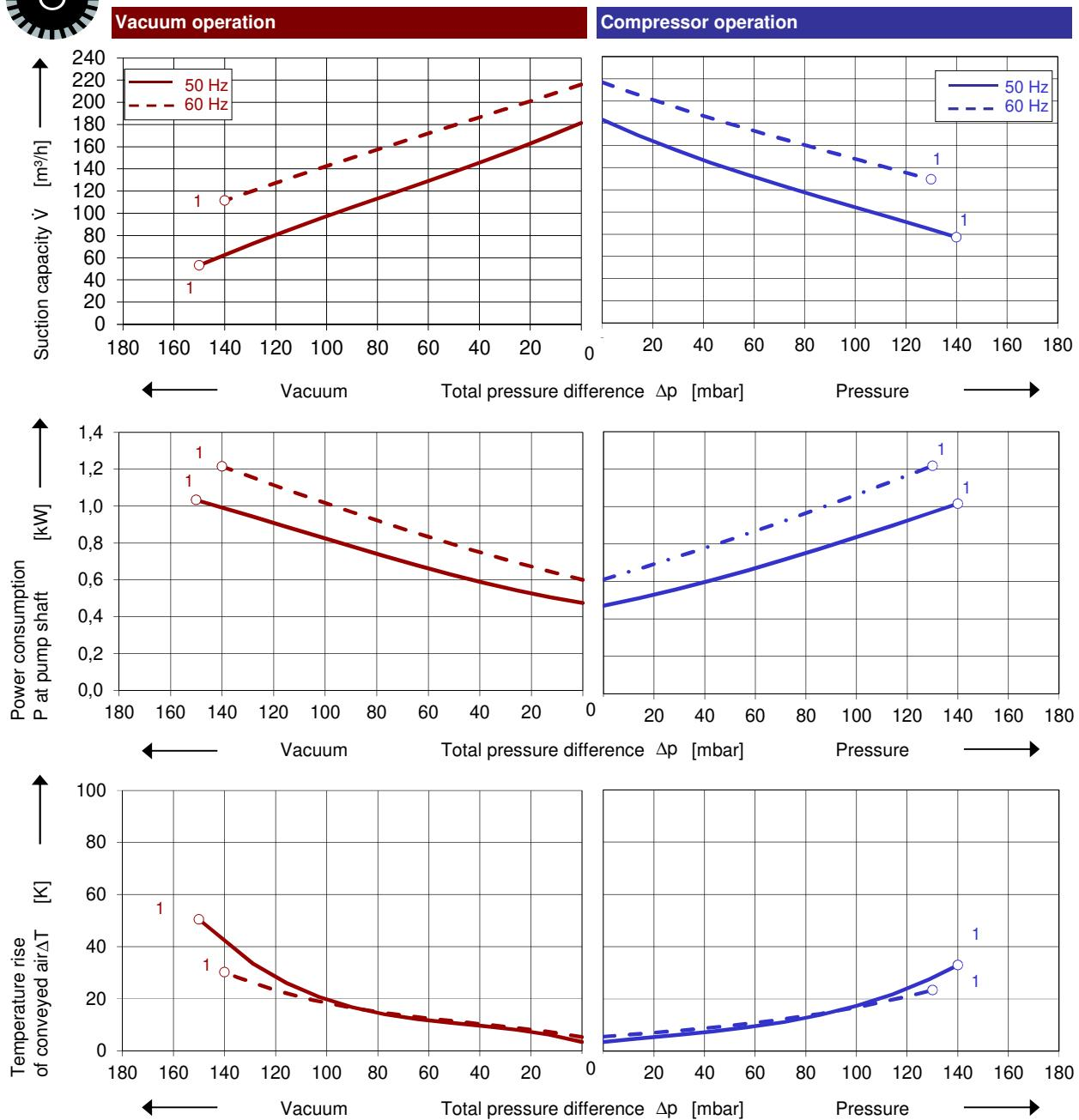
The performance curves are based on air at a temperature of 15 °C and an atmospheric pressure of 1013 mbar with a tolerance of  $\pm 10\%$ . The total pressure differences are valid for suction and ambient temperature up to 25 °C. For other conditions please get in touch with us.
