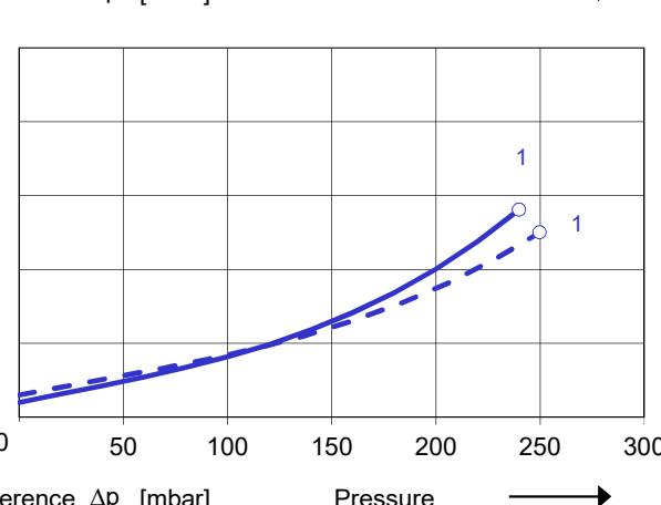
The performance curves are based on air at a temperature of 15 °C and an atmospheric pressure of 1013 mbar with a tolerance of  $\pm 10\%$ . The total pressure differences are valid for suction and ambient temperature up to 25 °C. For other conditions please get in touch with us.
