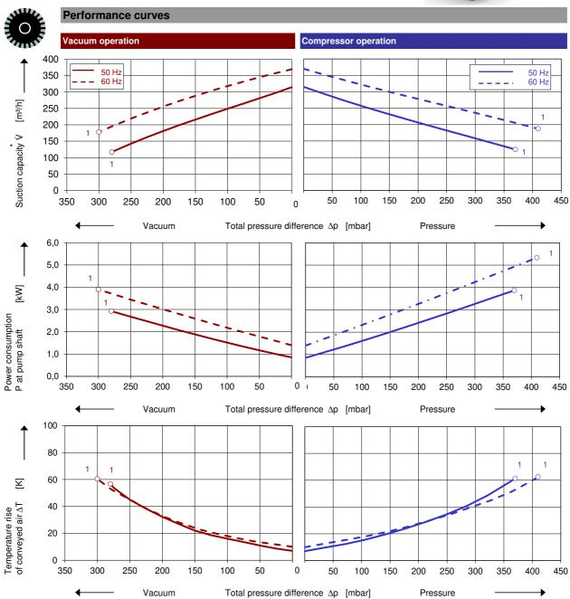
The performance curves are based on air at a temperature of 15 °C and an atmospheric pressure of 1013 mbar with a tolerance of  $\pm$  10 %. The total pressure differences are valid for suction and ambient temperature up to
